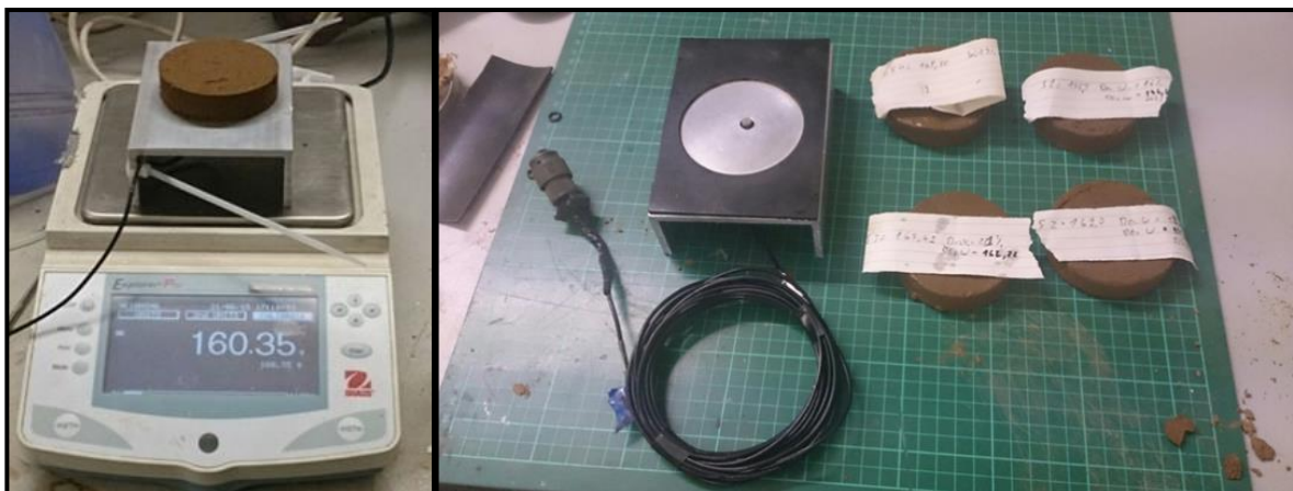
Figure 6.3 SWRC measurement set up using modified pore pressure transducer.
