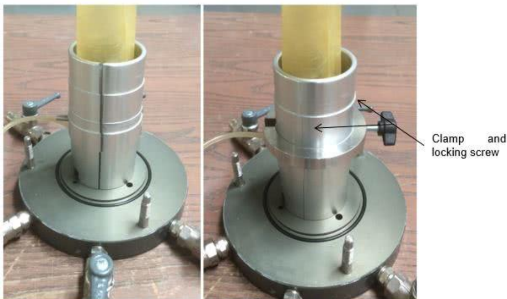
Figure 8.4 Schematic arrangement for soil sample placed on the pedestal.
