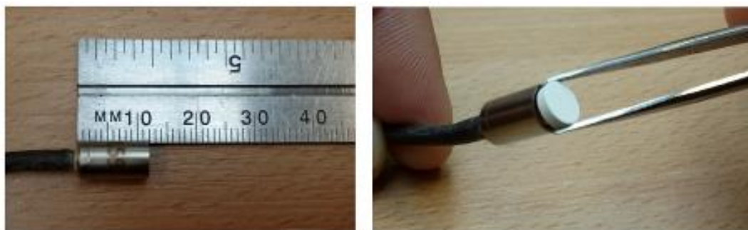
Figure 6.2 Pore Pressure Transducer (Druck PDCR81), fitted with a high air entry value porous disc.
