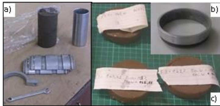
Figure 5.1 Sample preparation and trimming to desired size: a) sample core extruded after Proctor test; b) stainless still ring; c) soil specimens, size of 20/75 mm.
