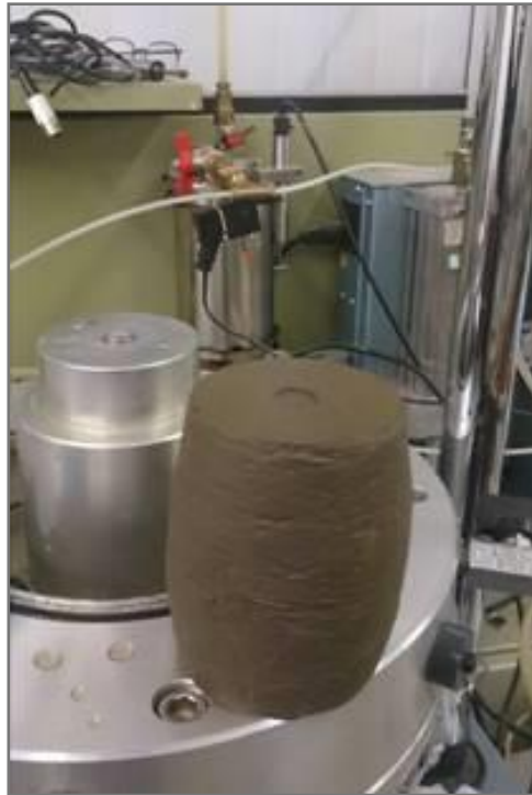
Fig 7.18 Bulging effect on samples at W_c(ac) = 20\% and 22\% after shearing.
